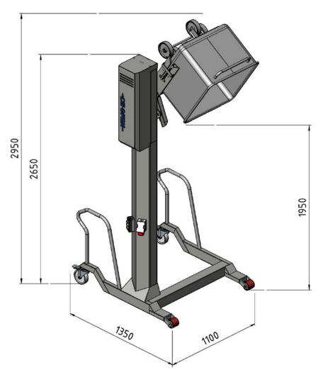
Weight of the KG lifting and tipping device: approx. 200 kg
